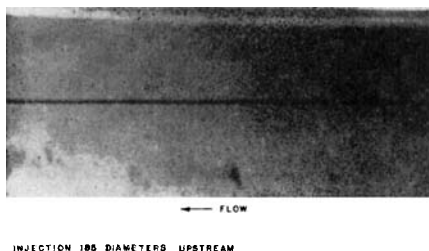
Fig. 7. Laminar flow, dye injection at tube center.
